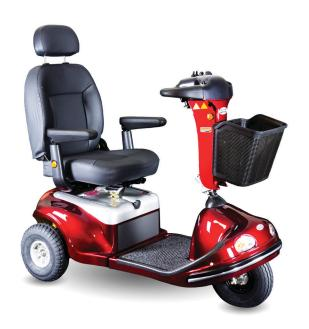
The Enduro XL3 is a heavy duty three-wheel scooter with a 500 lb. weight capacity. It has a delta style tiller which houses the controls for the lighting system, turn signals, wig wag and horn. It has a dual purpose wig wag which allows the user to push forward or pull back on the drive lever depending on dexterity for ease of driving. The unit comes standard with a 20in. seat that can accommodate most riders, and has swivel and recline features for added comfort and ease of use.
